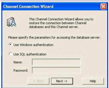
Indicate the mode you want to use when connecting to the SQL Server database that stores Channel information. You should select the same option you used during installation. This dialog box is part of the Connect Channel wizard in the Channel Server.
