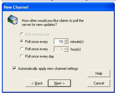
Set the default polling interval to be used for the Client computers to contact the Channel Server. The value you set here is used when computers are installed directly from the Console and for subscription files generated from this Channel. The values you set on this dialog box can be changed later by selecting **File** | **Client Settings**, and selecting the Polling tab.
